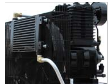
Air cooled after cooler Elite unit
