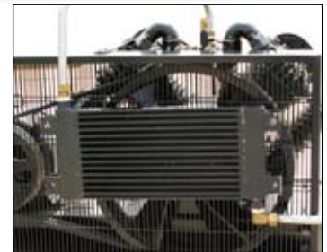
Air cooled after cooler Elite unit
